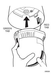
b. Line up the green and red tabs with the green and red labels. Push in on the tabs. Insert the side with the green tab, then the side with red tab. Continue pushing on the ends of the tabs until both sides click into place.
